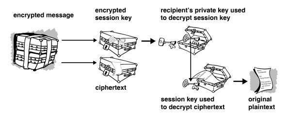
The combination of the two encryption methods combines the convenience of public-key encryption with the speed of conventional encryption. Conventional encryption is about 1,000 times faster than public-key encryption. Public-key encryption in turn provides a solution to key distribution and data transmission issues. Used together, performance and key distribution are improved without any sacrifice in security.
