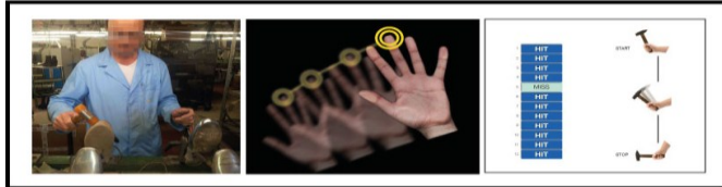
Figure 1. Left to right: (a) artisan hammering, (b) tracking the position of a hand, and (c) system performance with hammering.
