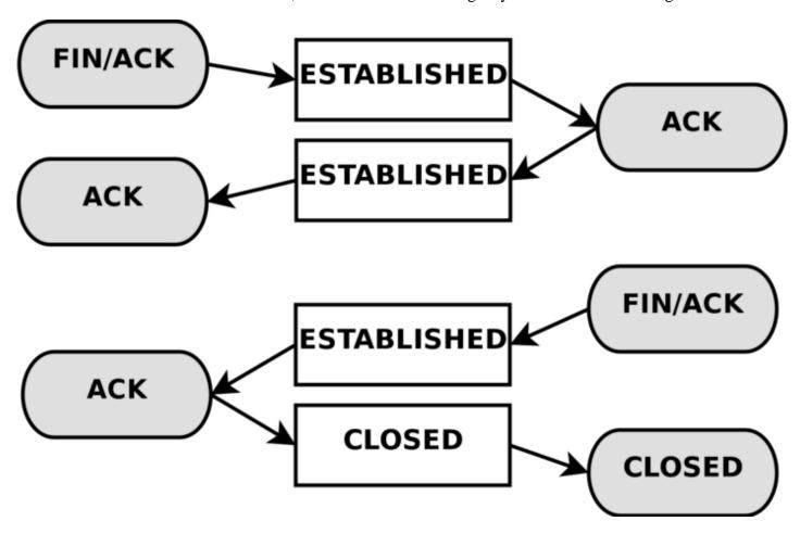
As you can see, the connection is never really closed until the last ACK is sent. Do note that this picture only describes how it is closed down under normal circumstances. A connection may also, for example, be closed by sending a RST(reset), if the connection were to be refused. In this case, the connection would be closed down immediately.
