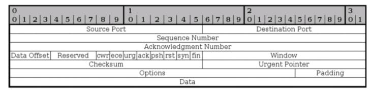
Source port - bit 0 - 15. This is the source port of the packet. The source port was originally bound directly to a process on the sending system. Today, we use a hash between the IP addresses, and both the destination and source ports to achieve this uniqueness that we can bind to a single application or program.
