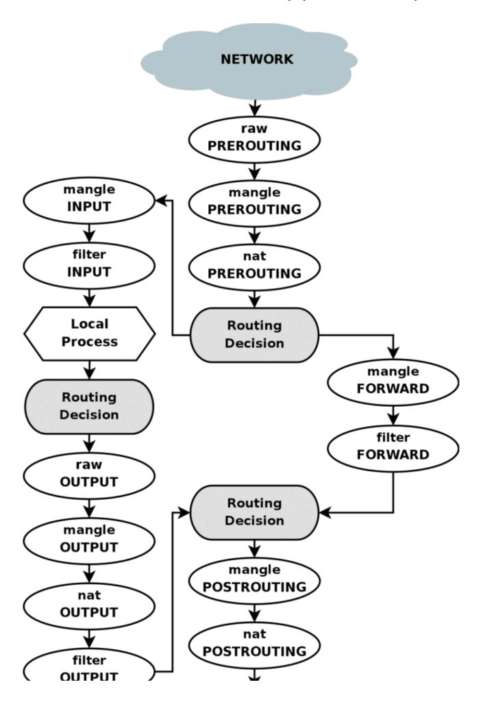
To clarify this image, consider this. If we get a packet into the first routing decision that is not destined for the local machine itself, it will be routed through the FORWARD chain. If the packet is, on the other hand, destined for an IP address that the local machine is listening to, we would send the packet through the INPUT chain and to the local machine.
