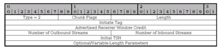
The INIT ACK chunk is sent in response to a INIT chunk and contains basically the same headers, but with values from the recipient of the original INIT chunk. In addition, it has two extra variable length parameters, the State Cookie and the Unrecognized Parameter parameters.
