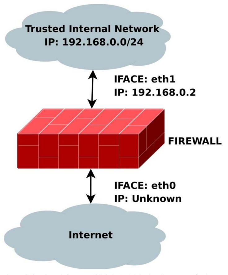
The <u>rc.DHCP.firewall.txt</u> script is pretty much identical to the original <u>rc.firewall.txt</u>. However, this script no longer uses the STATIC\_IP variable, which is the main change to the original rc.firewall.txt script. The reason is that this won't work together with a dynamic IP connection. The actual changes needed to be done to the original script are minimal, however, I've had some people mail me and ask about the problem so this script
