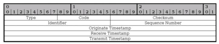
The timestamp type is obsolete these days, but we bring it up briefly here. Both the reply and the request has a single code (0). The request is type 13 while the reply is type 14. The timestamp packets contains 3 32-bit timestamps counting the milliseconds since midnight UT (Universal Time).
