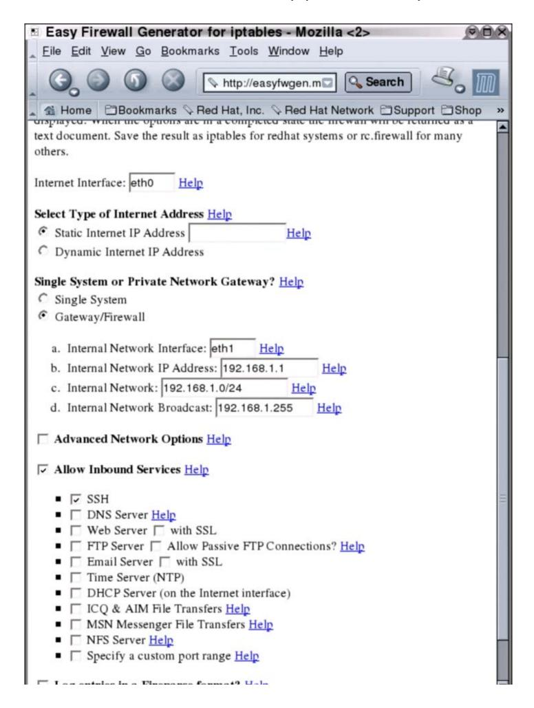
This screenshot shows one of the final stages of configuring the firewall script that is about to be created by the script. You can find more information, and a working version of the Easy Firewall Generator at <a href="http://easyfwgen.morizot.net/">http://easyfwgen.morizot.net/</a>.
