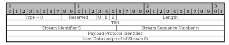
DATA chunks are used to send actual data through the stream and have rather complex headers in some ways, but not really worse than TCP headers in general. Each DATA chunk may be part of a different stream, since each SCTP connection can handle several different streams.
