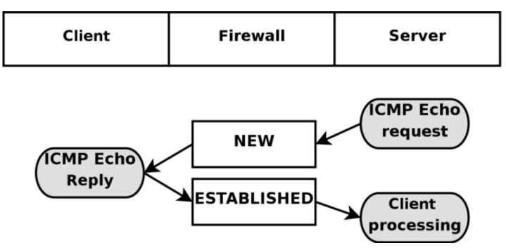
As you can see in the above picture, the host sends an echo request to the target, which is considered as NEW by the firewall. The target then responds with a echo reply which the firewall considers as state ESTABLISHED. When the first echo request has been seen, the following state entry goes into the <code>ip\_conntrack</code>.
