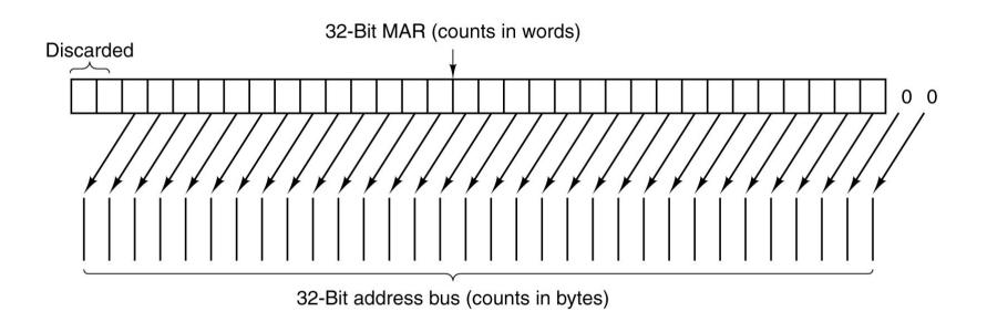
Mapping of the bits in MAR to the address bus.
