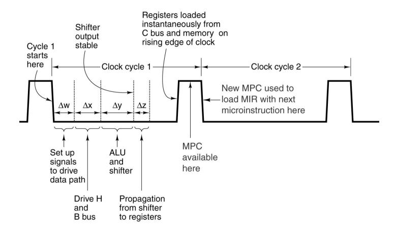
Timing diagram of one data path cycle.
