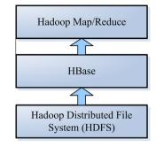
Fig. 6. Hadoop system architecture.
