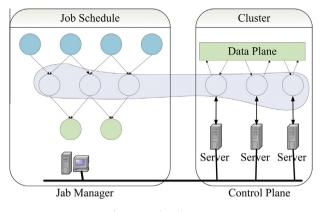
Fig. 9. Dryad architecture.
