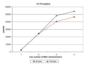
Figure 5. FTP total throughput with different MAC buffer sizes; user-AP distance = 10m, shadowing deviation = 9.
