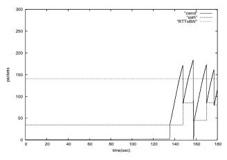
Figure 6. Measured TCP NewReno congestion window with max 3 retransmissions at the IEEE 802.11g MAC layer.
