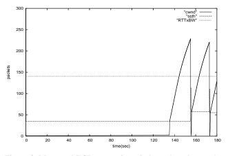
Figure 3. Measured TCP congestion window when the regular TCP NewReno and IEEE 802.11g are employed.
