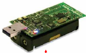
Hardware with USB interface for device programming
