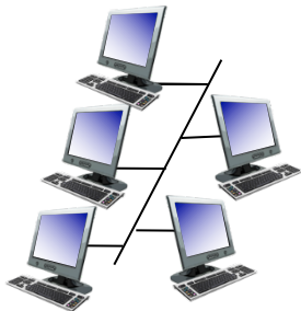
shared wire (e.g., cabled Ethernet)
