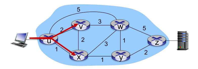
Q: what if network operator wants to split u-to-z traffic along uvwz and uxyz (load balancing)?A: can't do it (or need a new routing algorithm)
