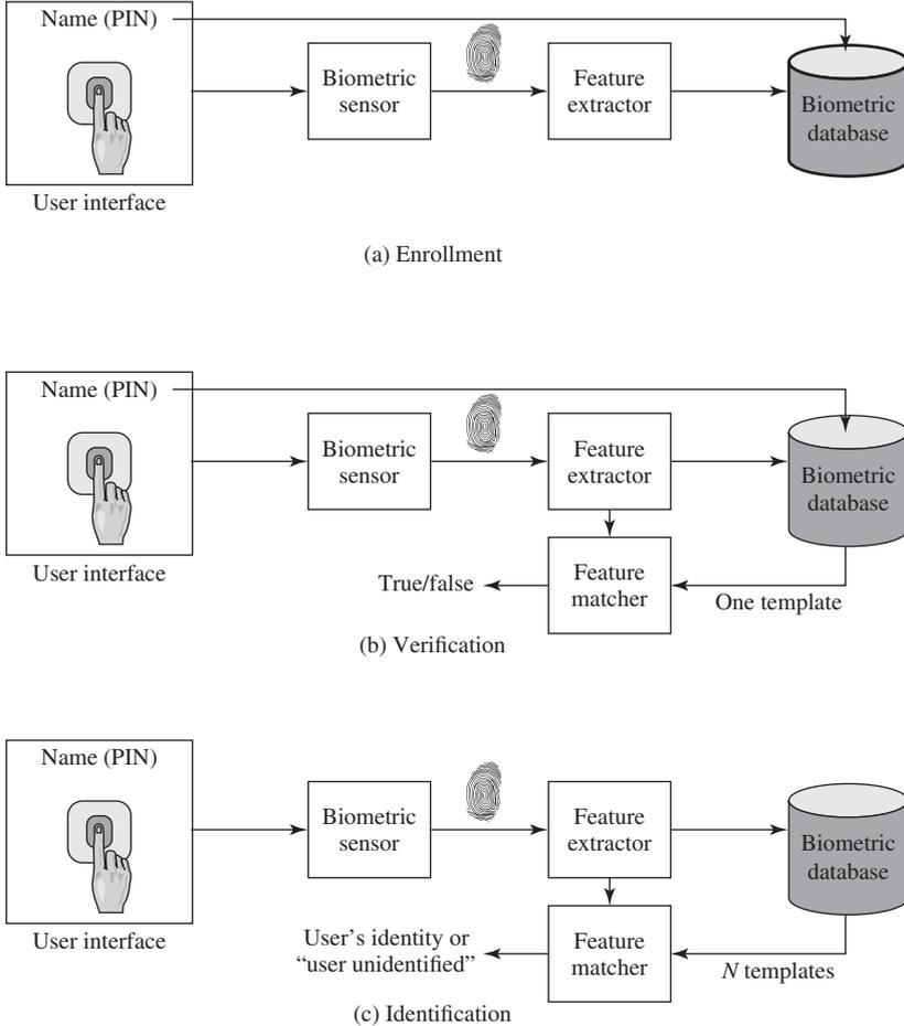
**Figure 3.8 A Generic Biometric System** Enrollment creates an association between a user and the user’s biometric characteristics. Depending on the application, user authentication either involves verifying that a claimed user is the actual user or identifying an unknown user.
