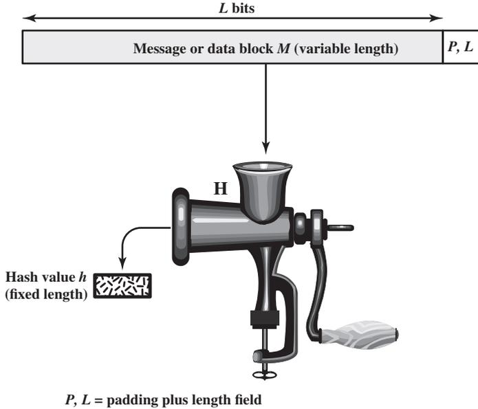
**Figure 2.4** Cryptographic Hash Function;  $h = H(M)$
