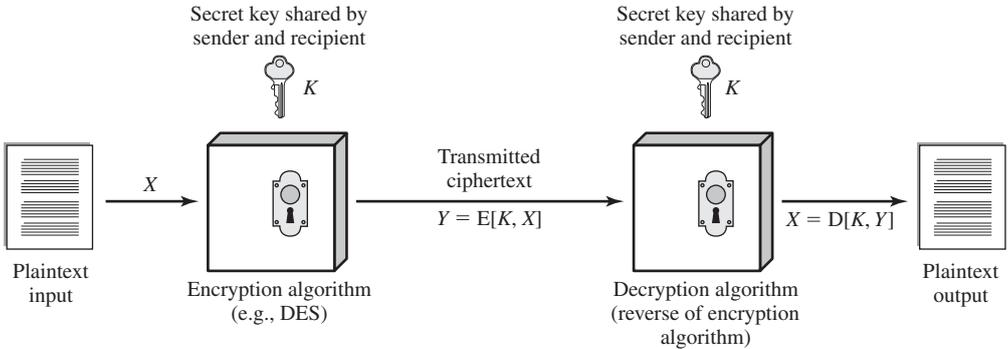
**Figure 2.1** Simplified Model of Symmetric Encryption
