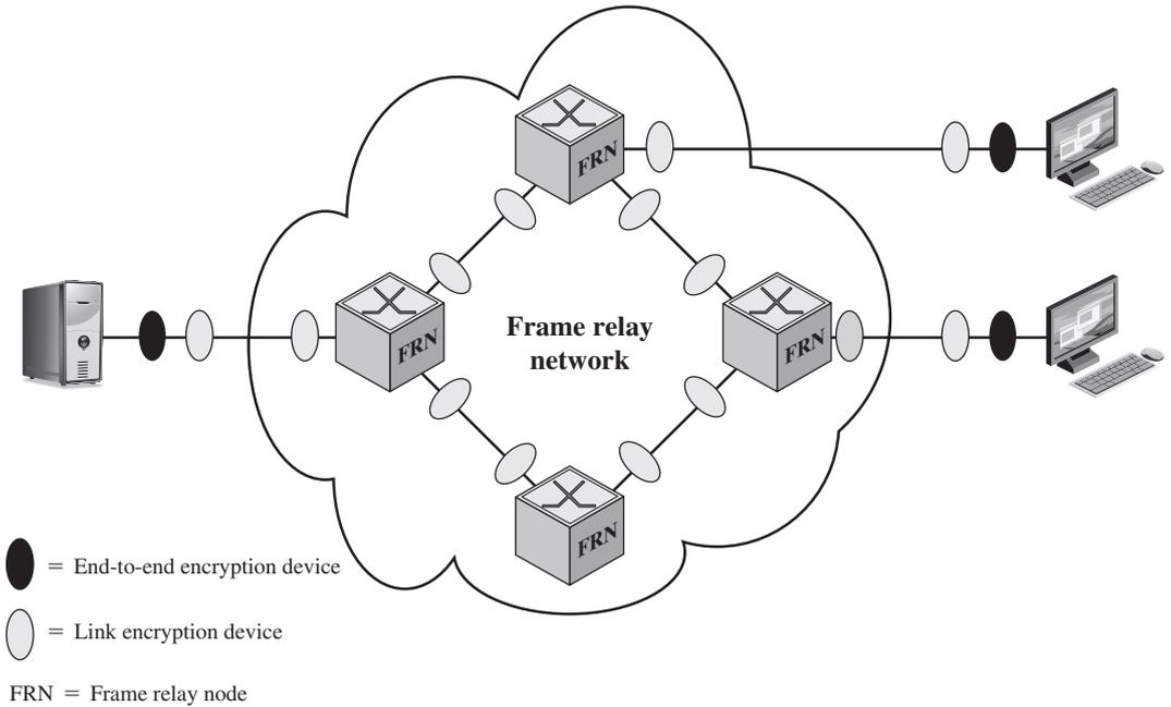
**Figure 20.9 Encryption Across a Frame Relay Network**
