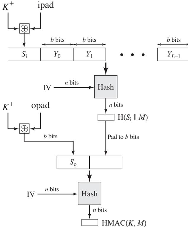
**Figure 21.4 HMAC Structure**
