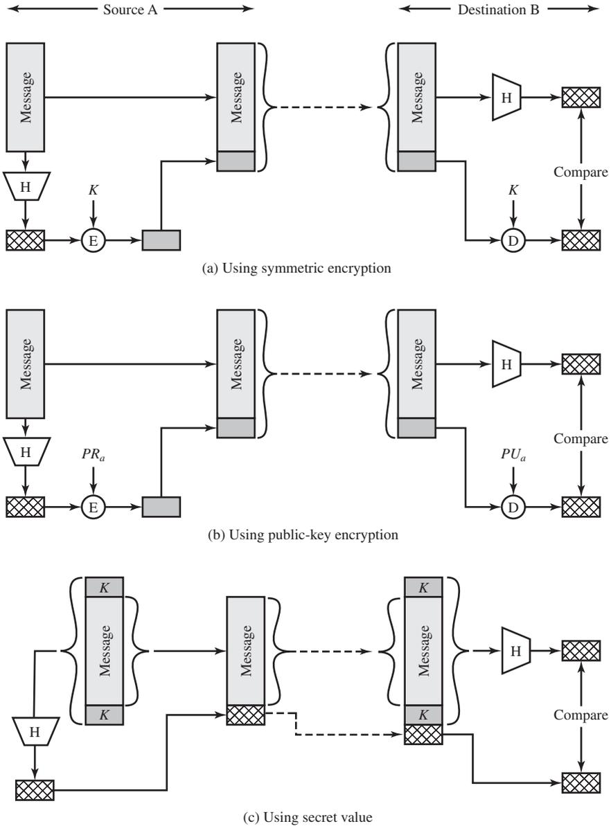
Figure 2.5 Message Authentication Using a One-Way Hash Function
