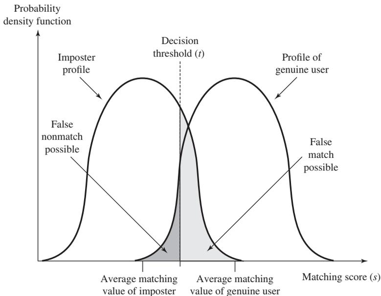
**Figure 3.9 Profiles of a Biometric Characteristic of an Imposter and an Authorized User** In this depiction, the comparison between the presented feature and a reference feature is reduced to a single numeric value. If the input value ( $s$ ) is greater than a preassigned threshold ( $t$ ), a match is declared.
