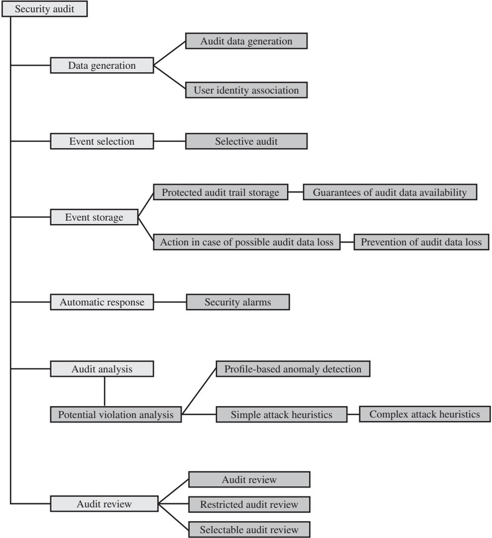
Figure 18.3 Common Criteria Security Audit Class Decomposition
