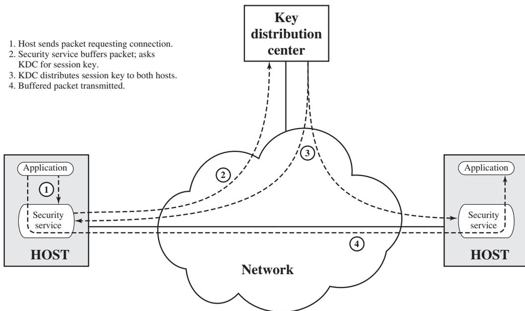
**Figure 20.10 Automatic Key Distribution for Connection-Oriented Protocol**
