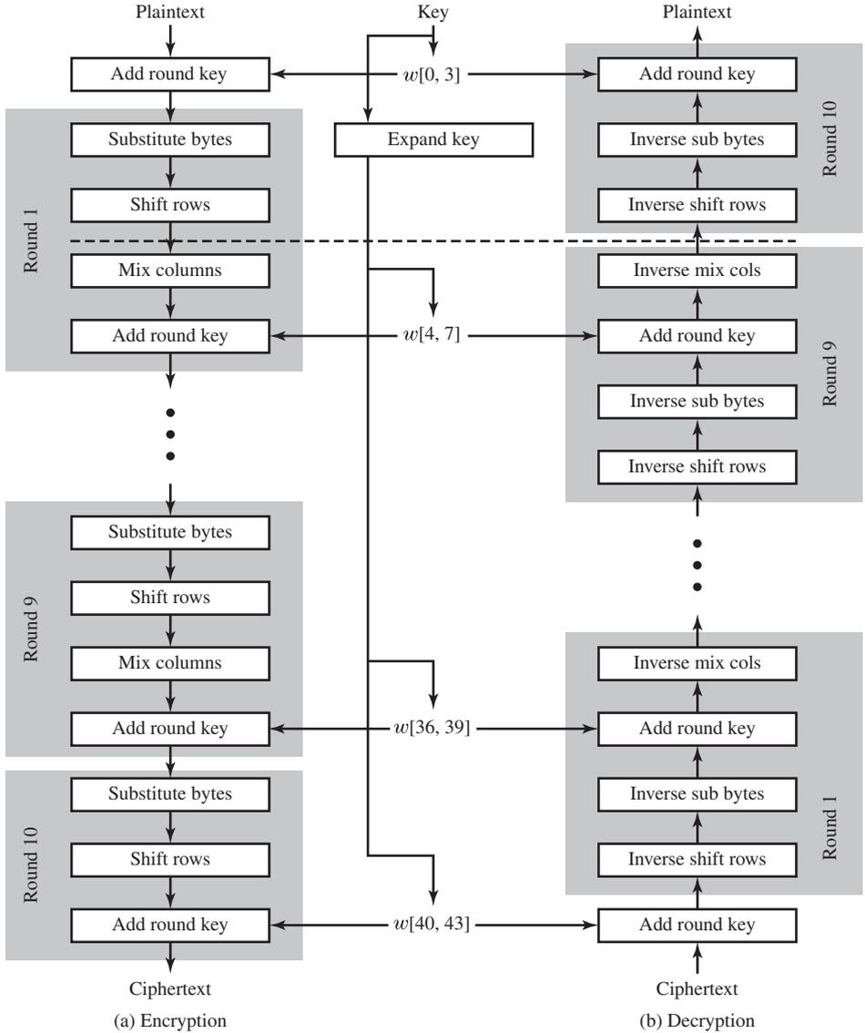
**Figure 20.3 AES Encryption and Decryption**
