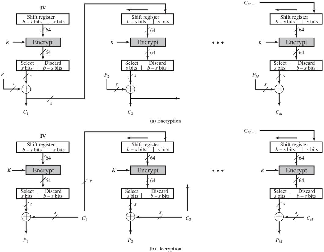
Figure 20.7  $s$ -bit Cipher Feedback (CFB) Mode
