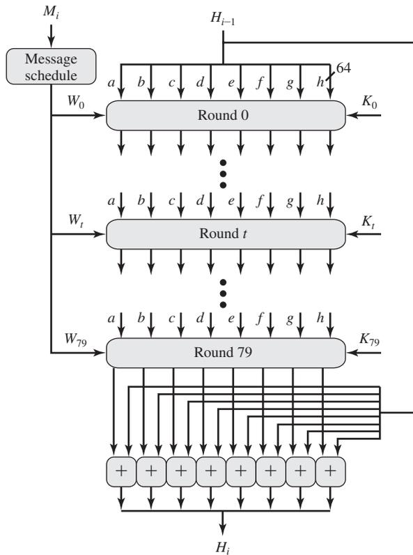
Figure 21.3 SHA-512 Processing of a Single 1024-Bit Block
