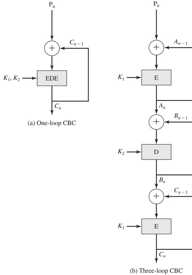
Figure 20.11 Use of Triple DES in CBC Mode
