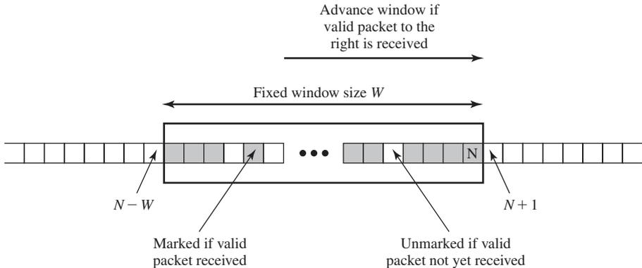
**Figure 22.9 Antireplay Mechanism**
