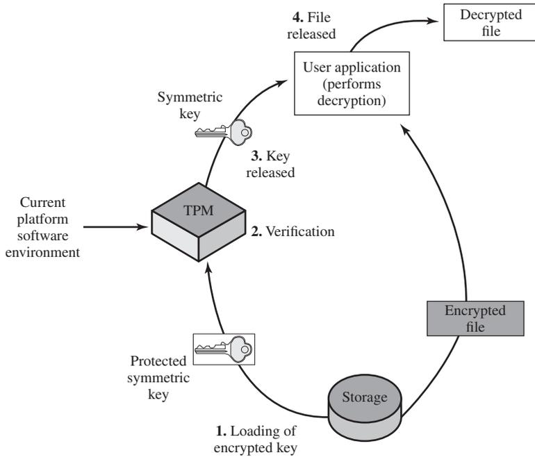
**Figure 13.12 Decrypting a File Using a Protected Key**
