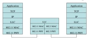
• The upper part of the data link control layer, the Logical Link Control (LCC) covers the differences of the Medum Access Control (MAC) layers needed for the different media
