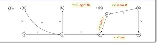
Communicating finite-state machines: Communication, locally  $proj(M, vendor) = \longrightarrow Q_4 \xrightarrow{w v?loginOK} Q_5 \xrightarrow{v c!request} Q_6 \xrightarrow{c v?pay} Q_3$   $c v?reject \xrightarrow{c v?reject} Q_3$
