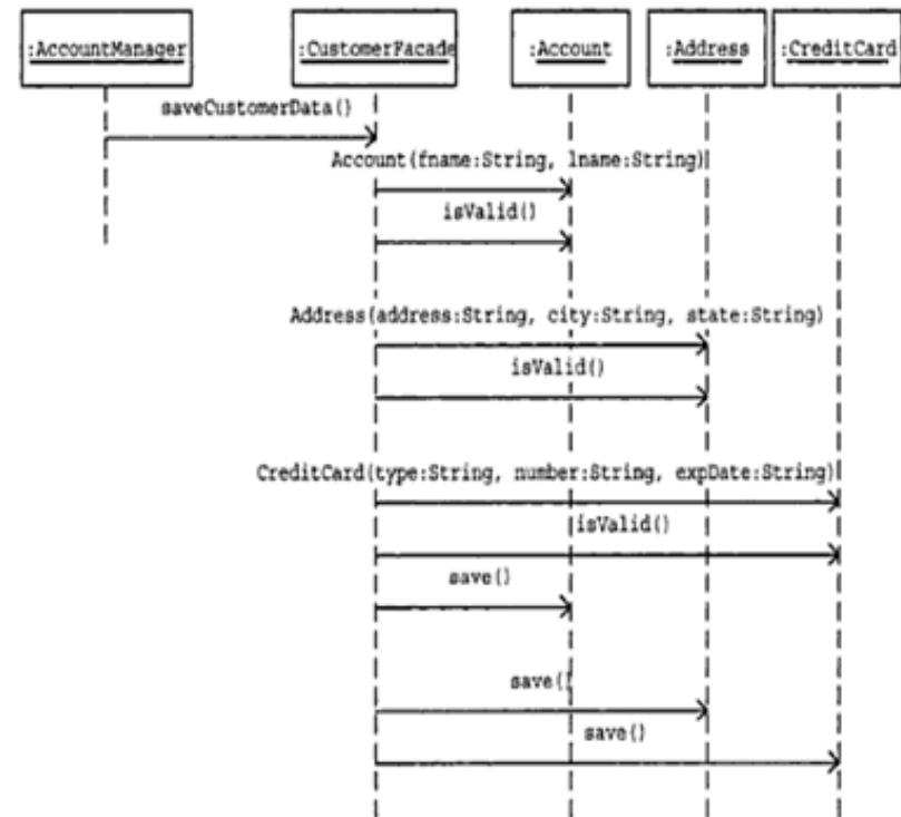
Figure 22.8 In the Revised Design, Clients Interact with the Façade Instance to Interface with the Subsystem
